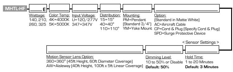
Hold Time - Time period for fixture remains at 100% output after motion is not detected Dimming Level - Fixture Light level after Hold Time (Disable - Fixture goes OFF after Hold Time)
